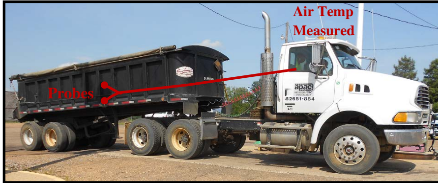
(a) Truck Showing Probe Locations and Cable
