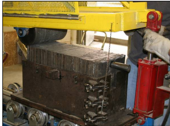
(b) Plates Over Mix During Compaction
