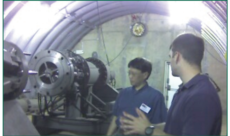
Blast load simulator (BLS) at the U.S. Army Engineer Research and Development Center used to conduct experimental blast tests. The BLS can simulate an approximate threat level of about 27,000 pounds of TNT at 184 feet.
