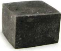
Fig. 8. A 1.378cm×1.1956cm×0.964cm parallelepiped shape cement paste sample.
