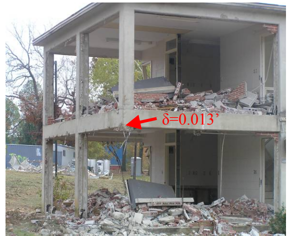
(c) corner sag measured in field test
