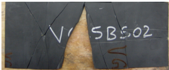
Figure 7. Real time image of 2.5% graphite platelet/vinyl ester specimen subjected to 120 psi peak pressure in shock tube [11]
