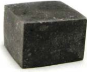
FIG.2— A 1.378cm × 1.1956cm × 0.964cm parallelepipedal shape cement paste sample
