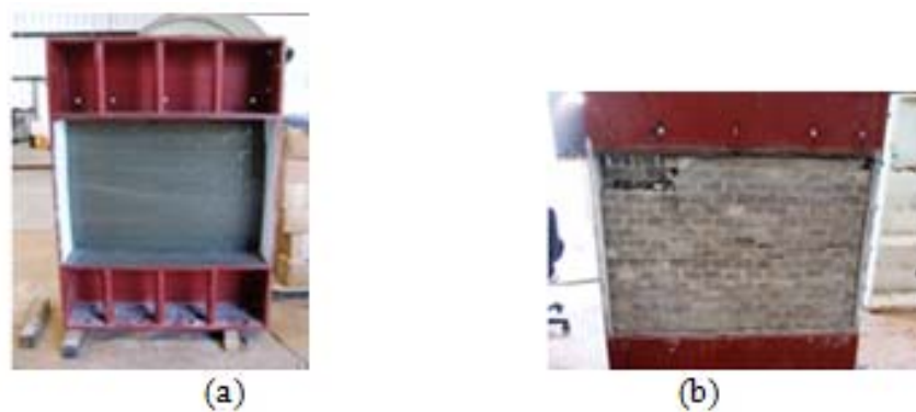
Figure 27: Wall #3 (a) back view after the blast event (b) front view after the blast event
