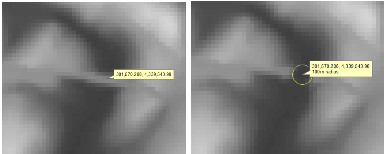
Figure 14. Removal of the bridge under the railroad embankment downstream of the Little Seneca Dam. Left: original DEM; Right: DEM after bridge removal.
