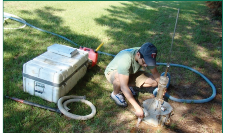
Measuring erosion coefficient using ASTM 6459-07 device.
