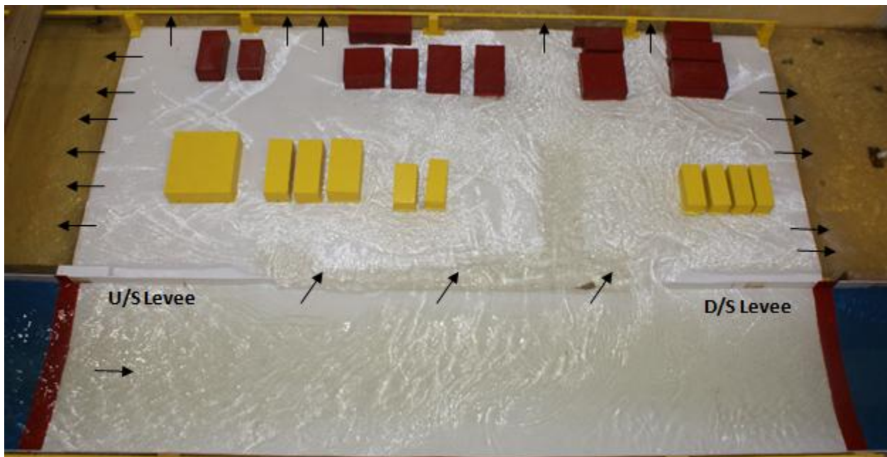
Fig. 1.2. Katrina model (arrows show water flow through the breach and outside the modeled neighborhood)
