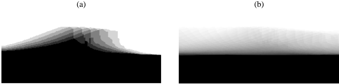
Figure 5. A portion of the average (a) five frames and (b) 48 frames for breaking waves over the sloping beach ( T = 1.6 s, H = 0.14 m and h = 0.4 m).
