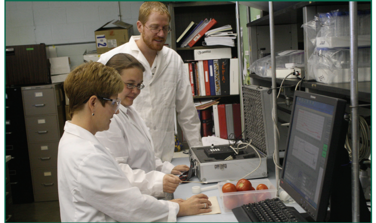
Project researchers examine a sample of tomatoes for Salmonella species using the prototype biosensor.
